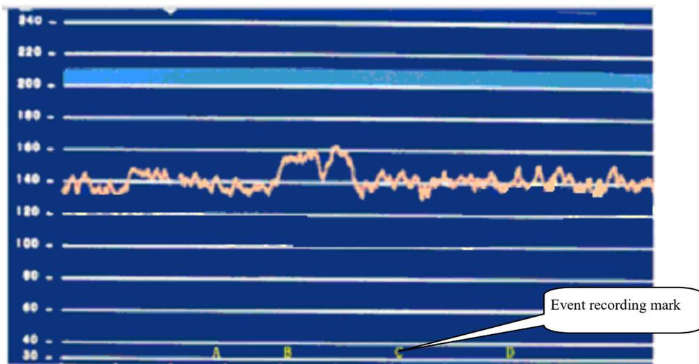
Fig.4-13 Event Recording Mark Display Bar
